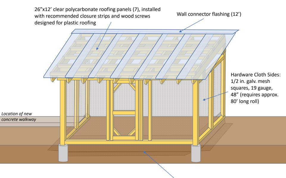
Buried Hardware Cloth Skirt: buried 10" & bent into L-shape, extending out 18"
